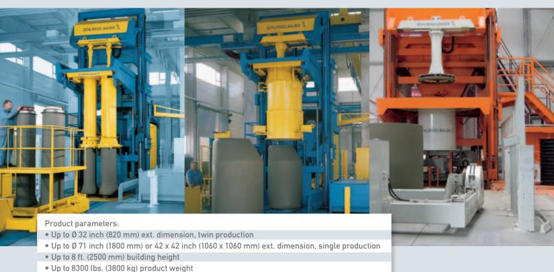
Production machine for reinforced and non-reinforced pipes, manhole components, road side channels and pipe connection parts.
