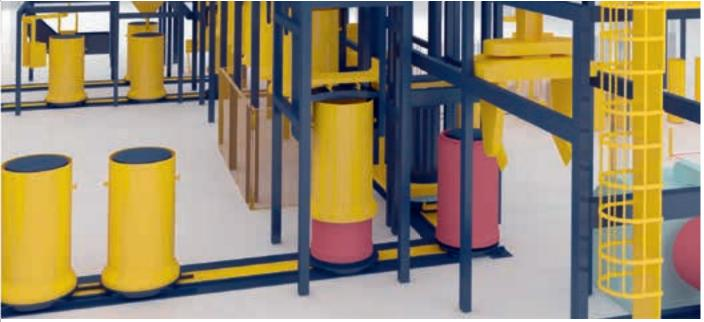
The ultimate contour of PERFECT PIPE is created by moulding the PERFECT LINER with pumped / fluid concrete. Different grades of concrete can be used. The dimensional stability of the inliner in the production process is in any case guaranteed by the inner steel core.
