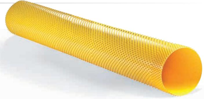
The PERFECT LINER is made of high-quality polyethylene (PE). This material is resistant to chemical attacks up to a ph-value of 1.0, abrasion-resistant and weldable.
