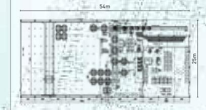
Layout of a PERFECT production system according to your needs, eg. with a production capacity of up to 100 manhole bases within 8 hours.
