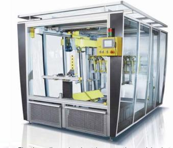
The three dimensional cutting operation applying hot wire cutting technique allows the production of custom made negative moulds/inverts.
