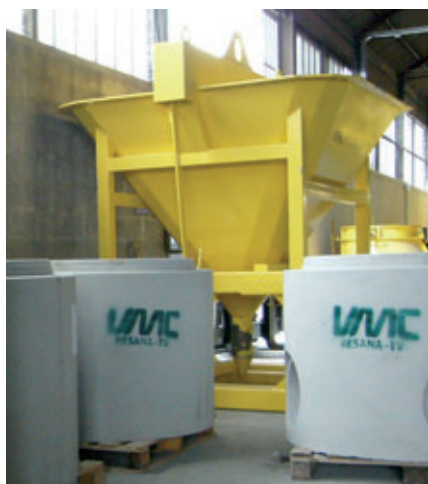
A concrete bucket brings only concrete of the class C60/75 into the casting moulds for the Perfect products.
