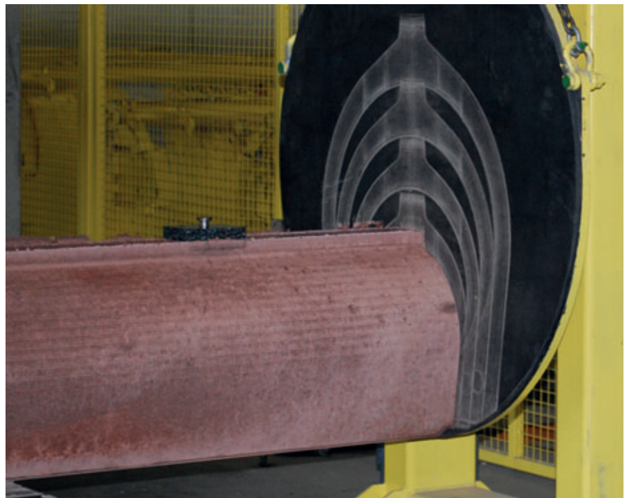
The wet-cast pipe made of self compacting concrete is subjected to a leak test in fully automated production before final approval.
