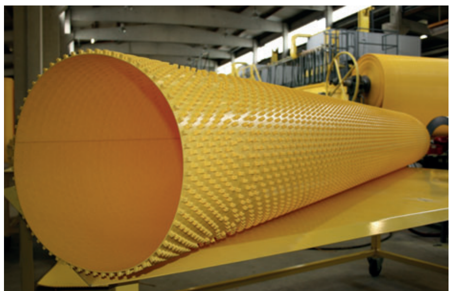
The HDPE liner is manufactured into cylinders and shows a wide range of anchors on the outside – for firm anchoring in concrete.
