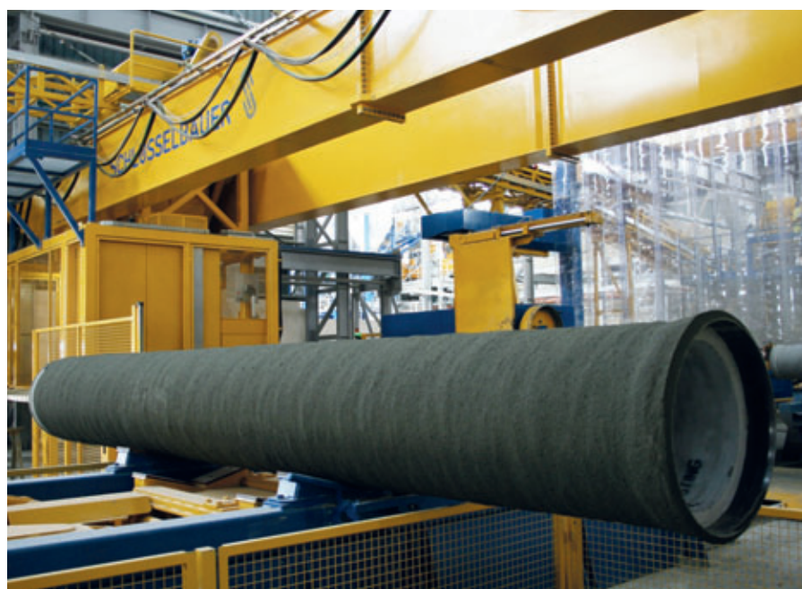
Pretensioned concrete pressure pipes with internal steel cylinders are absolutely impermeable and ideal for operating pressures of up to 25 bar.
