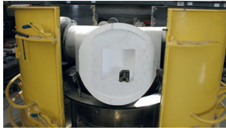
The assembled EPS negative channels are fixed in the steel mould using magnetic technology and secured from lifting.
