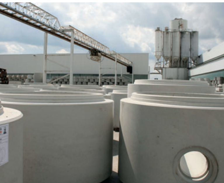
The central concrete plant with the Liebherr mixers produces the self-compacting concrete for the Grafe-Perfect manhole bases which is then transported to the production hall by truck mixer.
