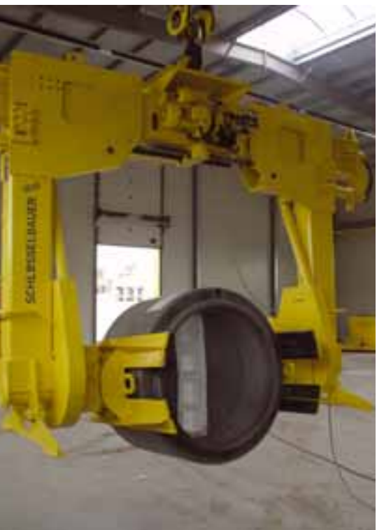
The Schlüsselbauer turning device turns cured manhole bases after removal of the moulds.
