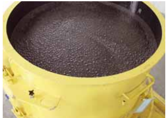
Manhole bases are manufactured using self compacting concrete, which is pumped into a mould by the Putzmeister pump.
