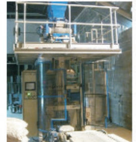
Continuous bagging machine of polyethylene/ polypropylene film
