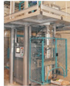
Continuous bagging machine of polyethylene/ polypropylene film
