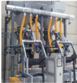
Pneumatic bagging machine for valve bags
