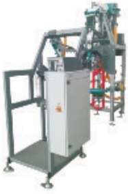
Pneumatic bagging machine for valve bags
