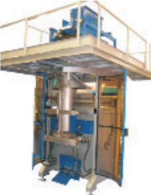
Continuous bagging machine of polyethylene/ polypropylene film
